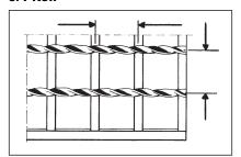
Distance between centre-to-centre of bearing bars and centre-to-centre of cross bars.
