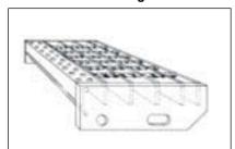
A visually accentuated member, perforated to provide serrations that reduce the risk of slip, which increases the load-carrying capability at its location and is welded to the leading edge of all treads and landings on stairs.
