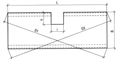
Max. diagonal deviation between D1 & D2 =  $\max$ . 0,005 x L Cutout dimensions i; k = + 8,0 mm; - 0,0 mm
