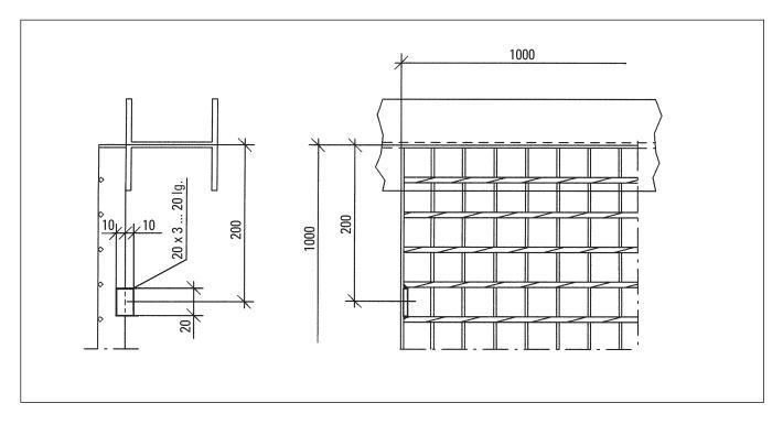
In accordance with the instructions of the professional associations, square gratings should be avoided where only two supports are provided, in order to ensure bearing bars are not running in the wrong direction following erection. Where it is not practical to avoid supplying square gratings, supports should be provided for all four sides of the grating, or arrangements should be made to prevent installation with bearing bars running in the wrong direction.
