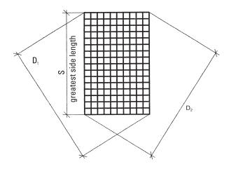
The difference between the measured diagonals D1 and D2 shall not exceed 0,010 x s, where s is the greatest side dimension.
