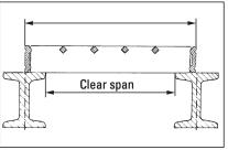
Distance between centre to centre of support. Clear span (effective span) is the clear distance between two supports.
