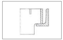
A cutout made to the lower part of bearing bars in order to reduce the level of the grating top to that of the surrounding area. A notched bearing bar should still be capable of sustaining the design load.
