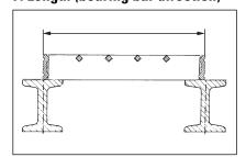
External distance of a metal grating in bearing bar direction. This size is termed length even if less than the width.
