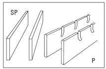
Bars bearing load lie parallel to each other between two grating supports
