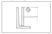
If an adjustment between height of grating and height of surrounding area is necessary, a deep binding bar is an option. Alternatively grating heights may be raised, by attaching other suitable sections to the underside.
