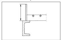
Binding bar projecting above the top surface of bearing bars by at least 100 mm (upstand).
