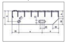
Plates provided with holes for bolting, welded to the ends of bearing bars in treads.
