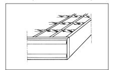
External distance of metal grating in cross bar direction. This size is termed width even if it is greater than the length.
