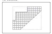
Straight or curved cutouts in metal gratings may be necessary to clear obstructions, plant or structural members. All cuts ends are bound after shaping.
