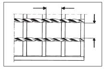
Clear distance between bearing bars and cross bars.
