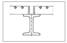
A structural section having a minimum clear distance of 30 mm available, to allow a minimum of 25 mm of bearing for bearing bars. Deviations may be permitted, providing suitable measures are taken to prevent excessive movement in the direction of bearing bars.
