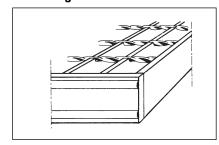
Bar or section to the edge of gratings, flush with the tops of bearing bars (in direction of bearing bar = binding along side; cross to bearing bar = cross binding).
