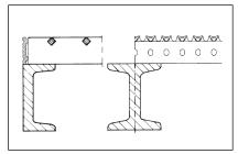
A structural unit provided beneath a grating that usually provides support.
